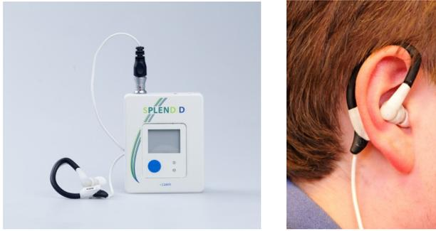
(a) The data-logger with the 3D accelerometer connected to the audio and PPG chewing sensor (b) Positioning of the chewing sensor
