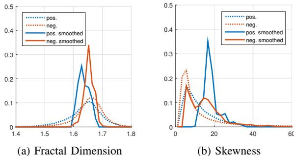
Fig. 3: Normalised (per-class) histograms for chewing (pos.) and non-chewing (neg.) windows of example audio features (original and 1-min smoothed).
